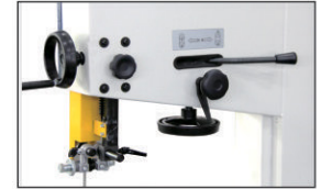
Blade quick release with hefty flywheel spring to help the saw withstand greater forces required for tensioning wide blades
