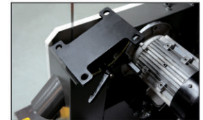
Oversize casting trunnions that lend solid foundation below and driven by gear for easy tilting
