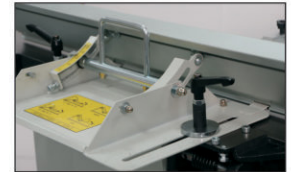
Centered controls and cam looking fence for quick adjustments
