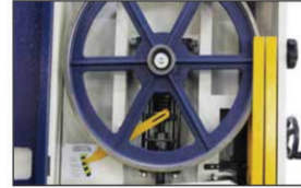
Reliable dual support blade tension system
