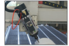
Italian HSD ATC 9KW Air Cool Spindle
