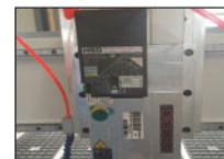
Italian HSD ATC 9KW Air Cool Spindle
