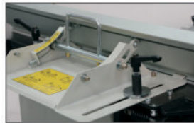
Centered controls and cam looking fence for quick adjustment
