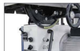
Gear drive table trunnion with quick locking mechanism
