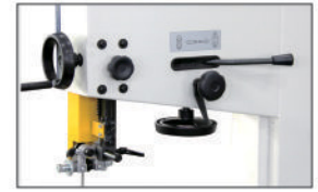
Blade quick release with hefty flywheel spring to help the saw withstand greater forces required for tensioning wide blades
